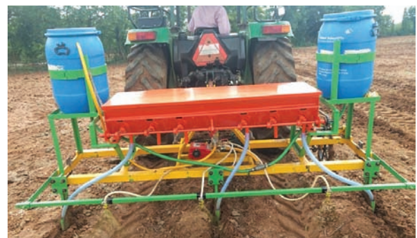
Planting through till-planter cum herbicide applicator designed for reduced and zero tillage
