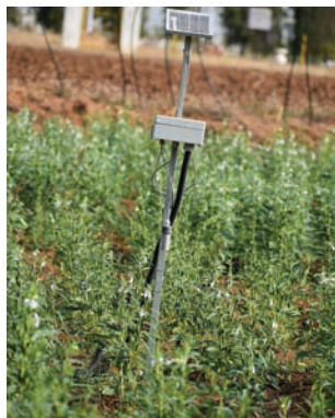
Soil moisture, temperature and atmospheric temperature and RH monitoring sensor in sesame field
